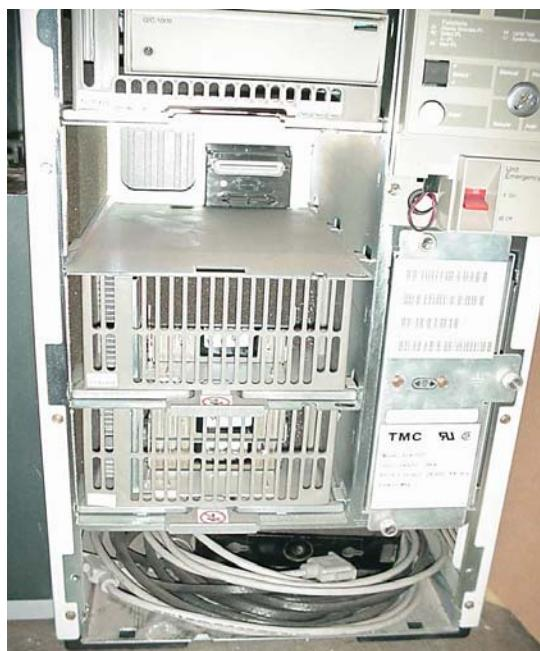
IBM AS/400 System with Drive Bays Exposed
