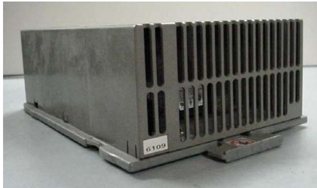
IBM AS/400 Drive Module: Front Side
